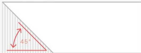
Overhangs less than 45° degrees, supports are needed
