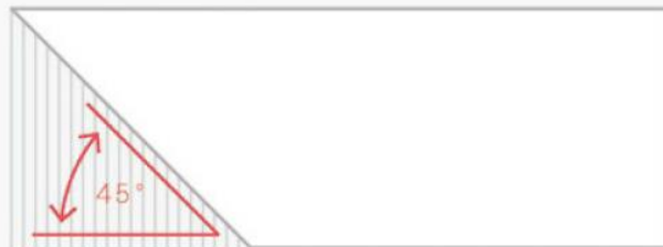
Overhangs less than 45° degrees, supports are needed
